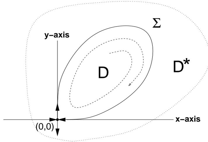
FIGURE 2. Attracting homoclinic loop in the plane. Inside the region bounded by the homoclinic cycle  $\Sigma$ , trajectories approach the cycle. Outside this region, trajectories eventually go away from the cycle.
