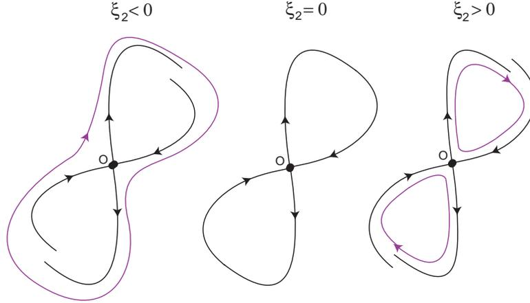
FIGURE 14. Bifurcations to periodic solutions near an attracting figure of eight cycle.
