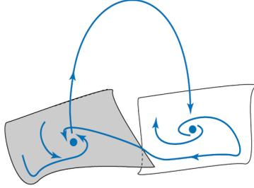
Figure 2: Bykov cycle: heteroclinic cycle associated to two saddle-foci of different types, in which the one-dimensional invariant manifolds coincide and the two-dimensional invariant manifolds have a transverse intersection.
